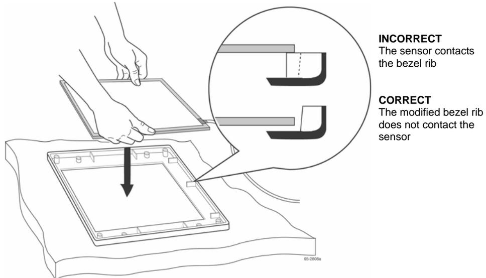
5. Carefully cut out a notch in each rib and cut back each fin that contacts the sensor.
