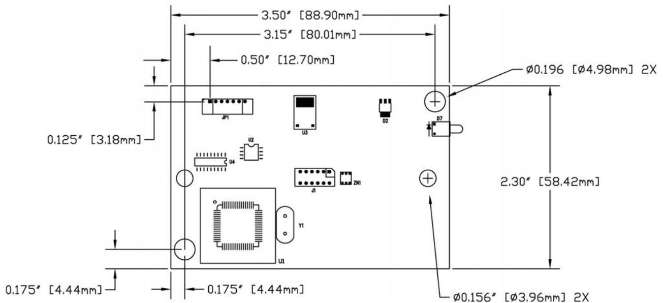
**Figure 2. EX II 7700 Dimensions**
