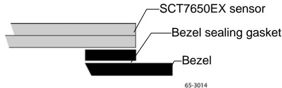
3. Remove the paper backing from the tape. Adhere a strip of gasket tape to each inside edge of the bezel opening. Align one edge of the gasket to the edge of the bezel opening. If the gasket overlaps the bezel edge, it will be visible from the front of the LCD. If the gasket is spaced away from the bezel edge, you will create a gap that can collect dust, liquids, etc.
