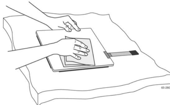
2. Apply strips of the double-sided acrylic foam tape (3M VHB 4956) around the perimeter of the LCD panel. Refer to the *Mechanical Considerations* section in Chapter 2 for additional details.
