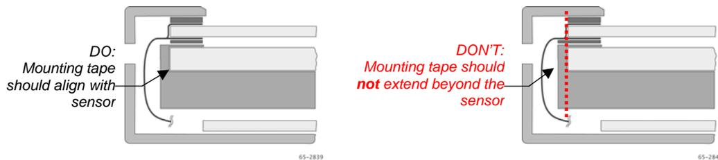
**Note:** 3M VHB acrylic foam tapes (Product Numbers 4956, 4956F, or 4979F) are well suited for this purpose. These tapes were chosen for their thermal properties. The typical Thermal Coefficient of Expansion for these tapes is  $1.8 \times 10^{-4}$  mm/mm/°C.
