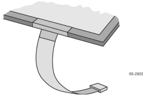
3. Remove the paper backing from the double-sided tape on the LCD panel.
