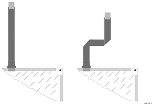
The sensor flex tail is designed to be flexible, and it may be creased *once in a single direction*, in multiple locations along the flex tail and then secured in position with a light adhesive tape. Avoid angular creases (45°) to the flex tail directly in the area of the bond and tape strain relief.
