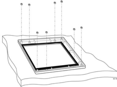
3. Align the screw holes (or tabs) over the temporary post. Each LCD hole/tab must rest on top of the spacer and washer above the bezel screw hole.
