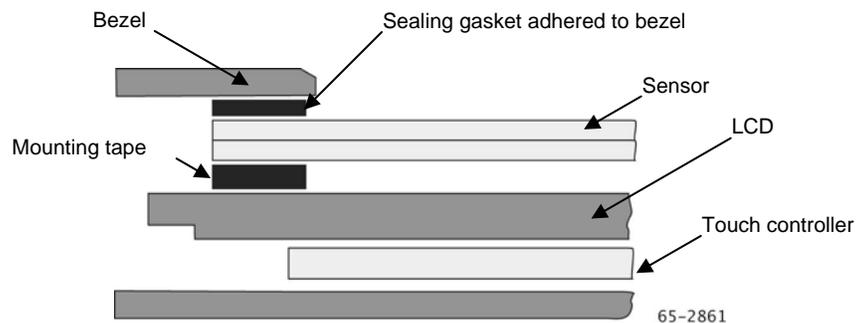
Remember to choose a gasket material with recommended thickness of 3 mm or greater before compression and attach it to the inside of the bezel opening.
