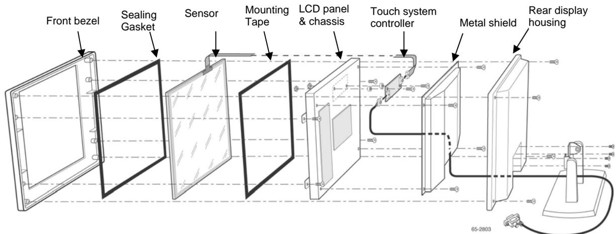
You can install a 3M™ MicroTouch™ SCT7650 sensor on most displays. Although each particular display may have some unique integration considerations, the basic installation process consists of the following steps:
